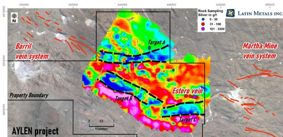
***Figure 1: Drill targets defined by ground magnetic surveying and previous rock sampling results at the Aylen Project, Santa Cruz Projects.***
