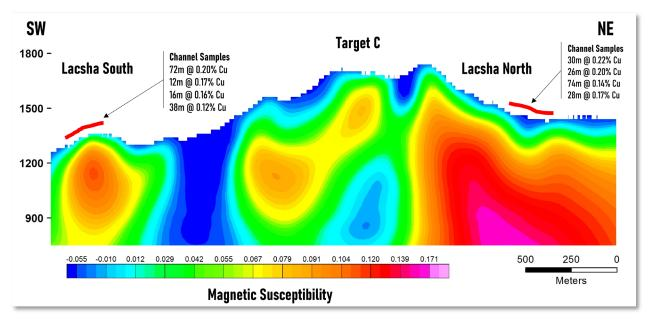
Figure 2 Inversion model NE-SW section showing high magnetic anomalies just below surface, interpreted to be the potassic core of a porphyry system.
